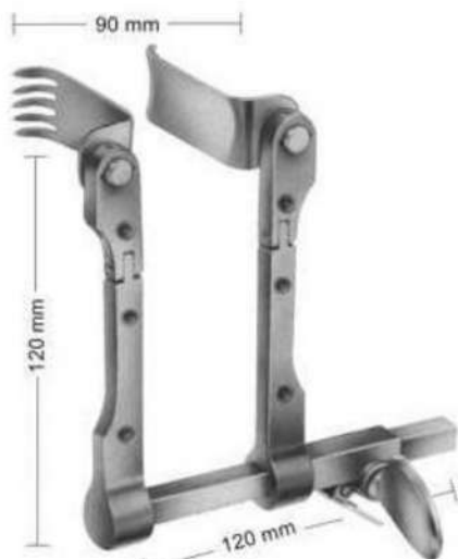
03-5387 CASPAR Retractor, adjustable, consisting of: 5 medial blades (03-5389 - 03-5393) 5 Lateral blades. (03-5394 - 03-5398) and the retractor only By Reversing the Screw, The Retractor Can be Used From Both Sides
